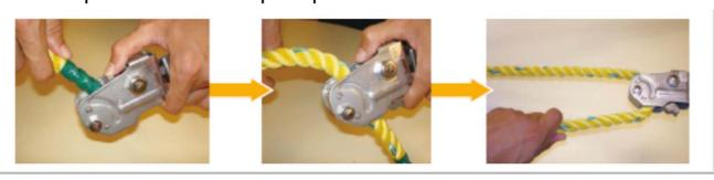
Press down on the teeth profile to release rope.
